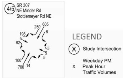
Figure 11. Future (2028) With-Project Traffic Volumes Aligning Bond Rd NE (SR 307)/Stottlemeyer Rd NE/Minder Rd
