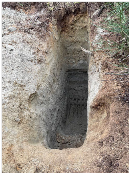
Photograph 3: Exploration pit EP-16 with Vashon recessional outwash fine sand and no groundwater seeps.
